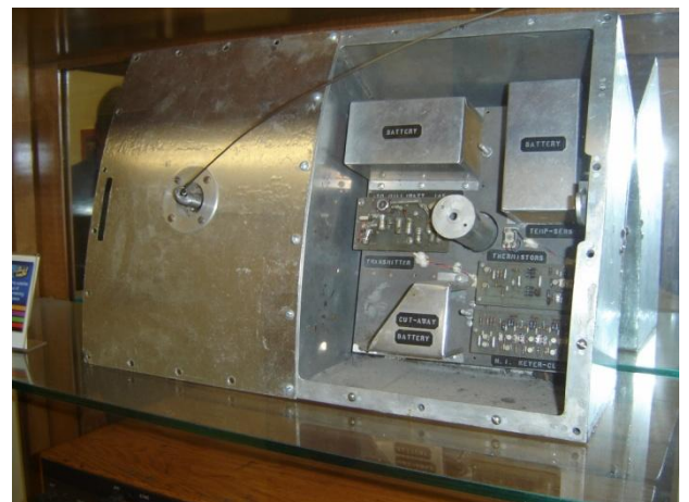
A close-up of the inner workings of OSCAR-1 (Courtesy: Author)
