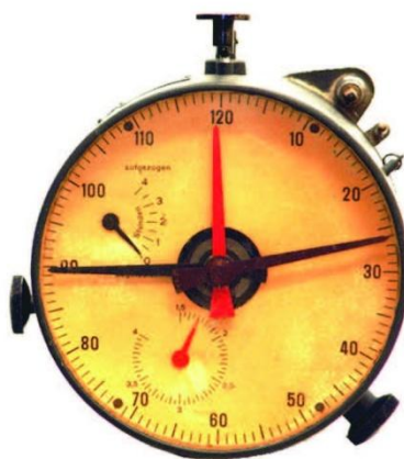
The X-Gerät 'bombing-clock' measured the time to fly between two crossbeams to determine the bomb release time. (Horst Beck Collection, photo Frank Dörenberg, N4SPP/F4WCN).
