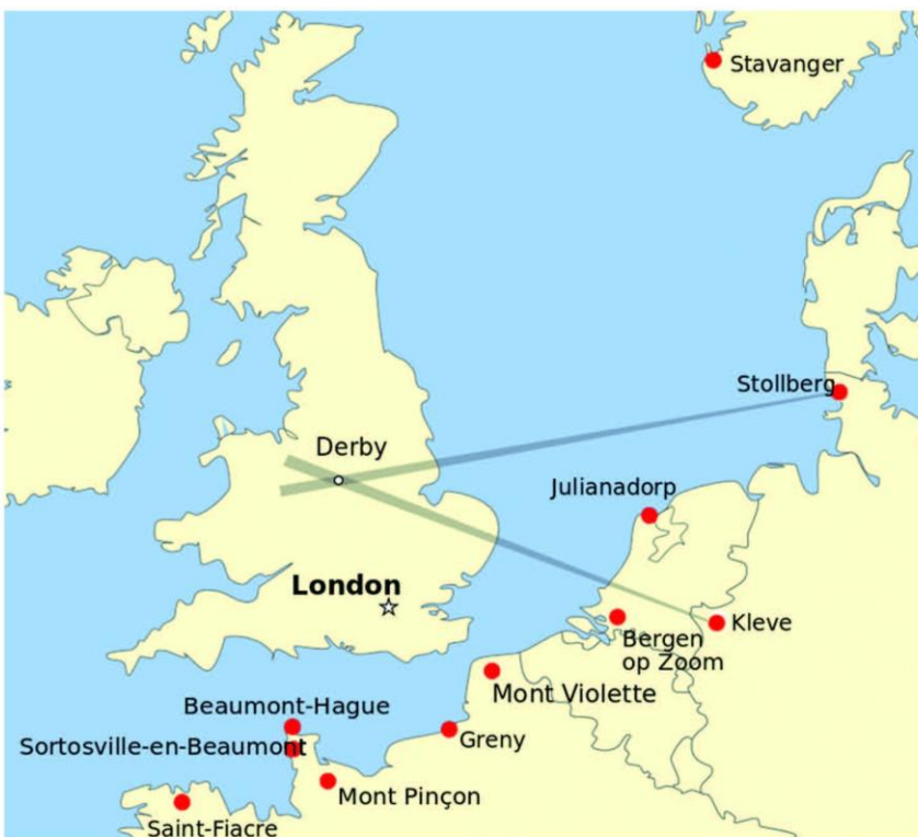
The Knickebein beams from Kleve and Stollberg could be directed to intersect over targets such as the Rolls-Royce aero-engine factory at Derby. (Image: Dahnielson/cc by-sa 3.0).
