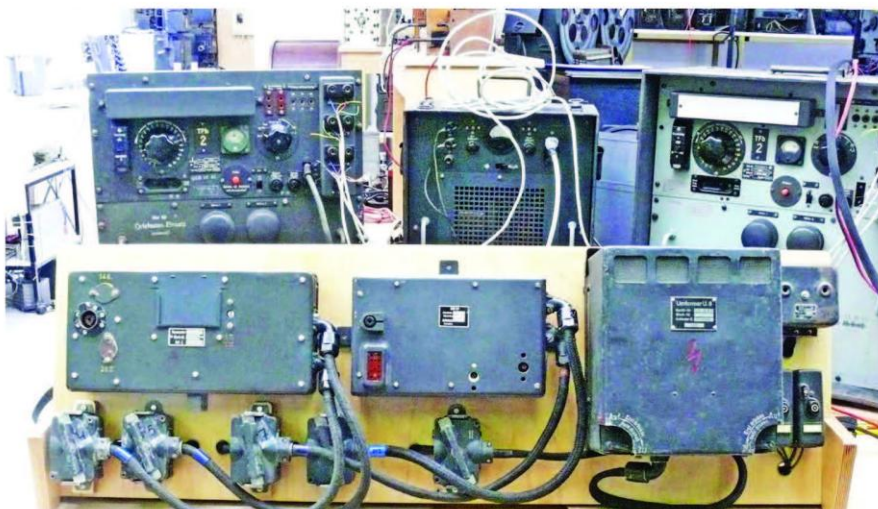
Restoring an aircraft Knickebein system (foreground). Left: EBL2 signal processing unit; Middle: EBL3 superhet beam receiver; Right: U8 210V HT rotary converter. (CDV&T and Hans Goulloze).
