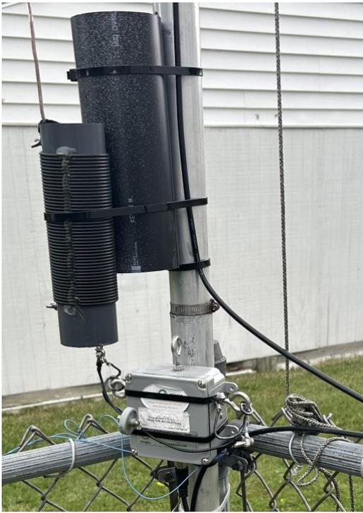
The feedpoint at my aluminum mast. The coil (20uH): 2" PVC form, 45 turns of 16ga antenna wire. The large (3") PVC is a spacer for less coupling to the mast. The matching unit is a Balun Designs 4:1 balun. I used a 3.5kV 220pF doorknob capacitor across the feed.
