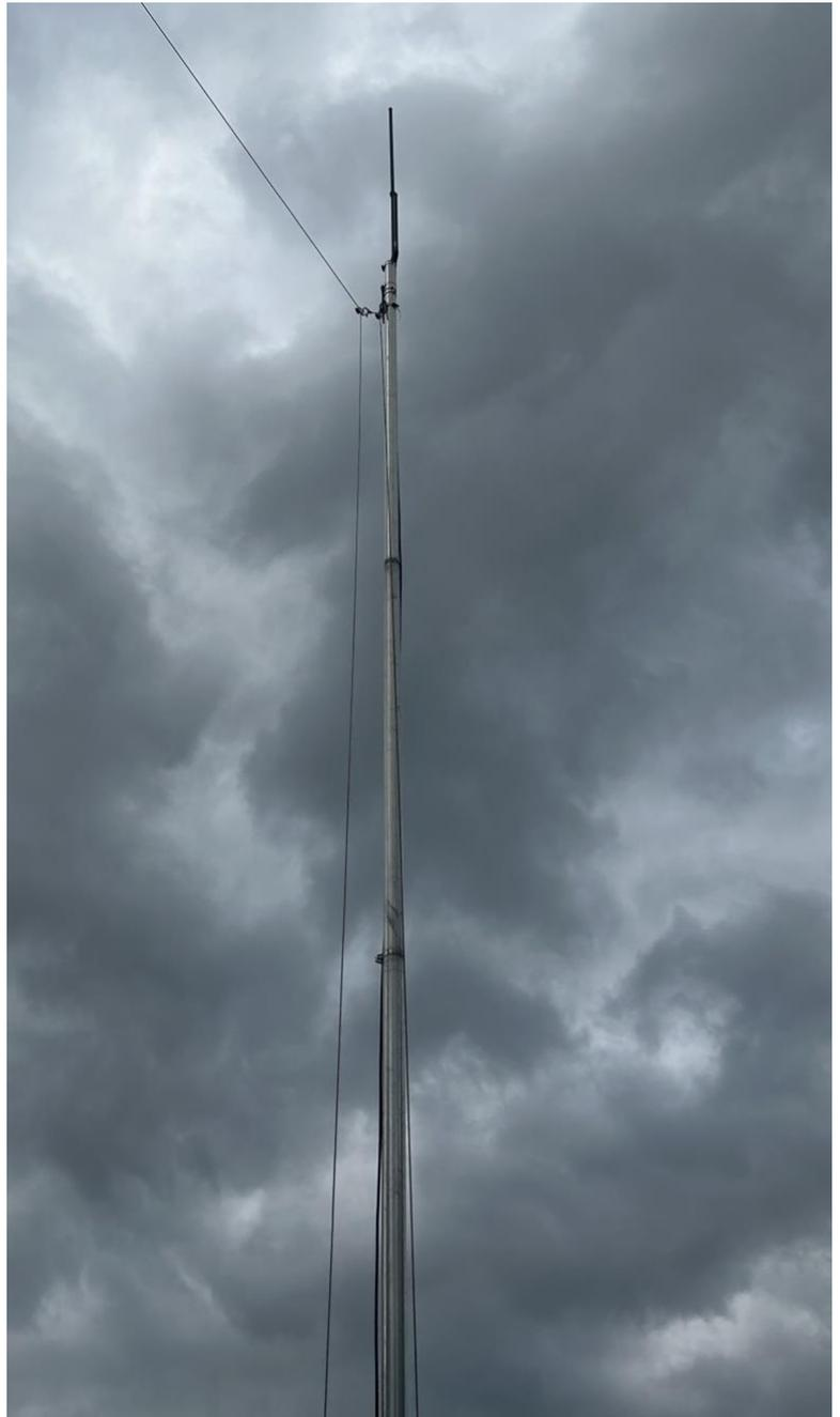
I tried many combinations of wire length, inductance, capacitance and placement of the coil. A “normal” inverted L uses 165’ to 175’ of wire. The longest I could do (without dropping it to the ground) was 137”. I tried that length first, then trimmed it back for the best results. Each time I trimmed the wire, I tried combinations of L/C/coil placement. It was an iterative process... and slow.
