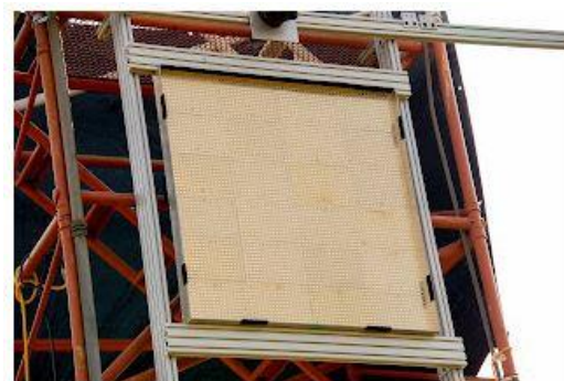
A "rectifying antenna" connected to the receiving antenna converts the 10-GHz RF energy into electricity. (NRL Photo by Gayle Fullerton)
