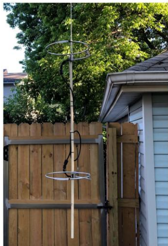
Figure 1- Stacked 2M halos with phasing harness. When raised on a rope over a tree limb it's around 45 feet above ground.
