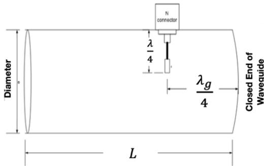
Most of the time we will be using only one can for our excited waveguide antenna. We say they are excited because we insert a small radiator into the waveguide to provide the RF energy. Our designs will look like Figure 7 where our signal is connected to the N connector.
