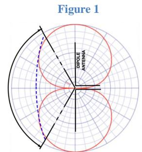
You can see that to increase the aperture angle you will need a smaller F/D ratio. This reduction in F/D will make your dish flatter. Even with the best possible F/D ratio, it is also easy to see this antenna subsystem is not very efficient with often over fifty percent of the radiation (radiation sent away from the dish) wasted.
